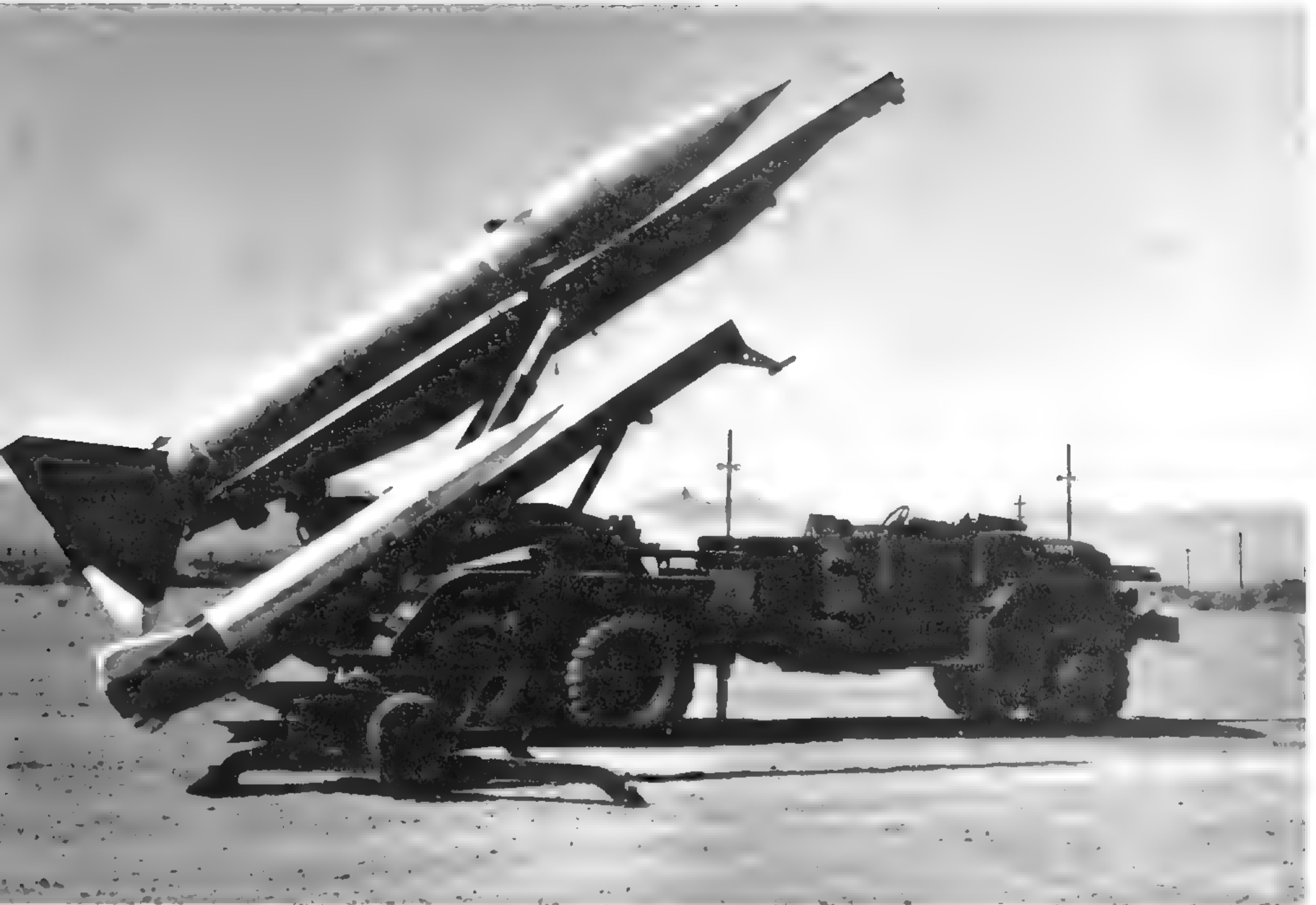
The M386 was built on the M139F chassis. Its launch rail was noticeably shorter than that of the M289, and the truck lacked the A-frame brace on the front bumper. (Photo courtesy of Patton Museum)
